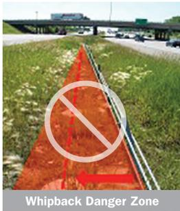
If a collision occurs on a curve, this places additional tension and pressure on the cable and may result in the cable releasing and whipping toward the inside of the curve. All personnel should be positioned outside of the curvature during the recovery of a crashed vehicle.
